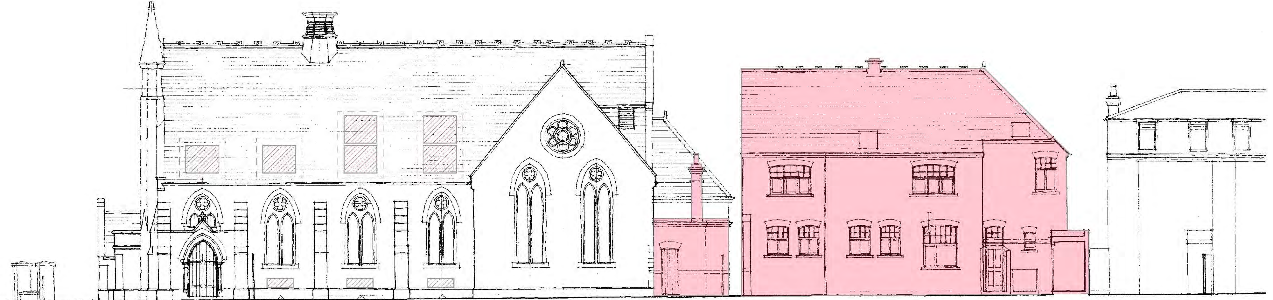
Demolitions North Elevation
